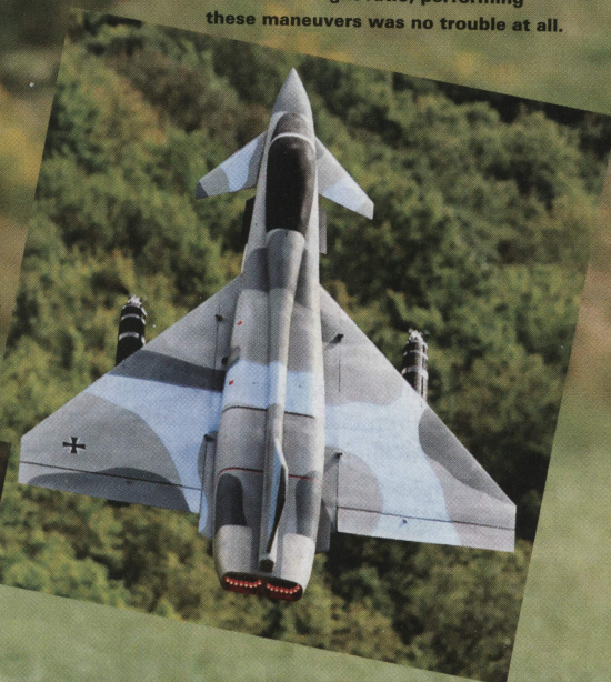
Adam Woodworth's demonstration flight showed off the slow and low flight capabilities of his Eurofighter. With a length of 106 inches and a 2:1 thrust-to-weight ratio, performing these maneuvers was no trouble at all.
