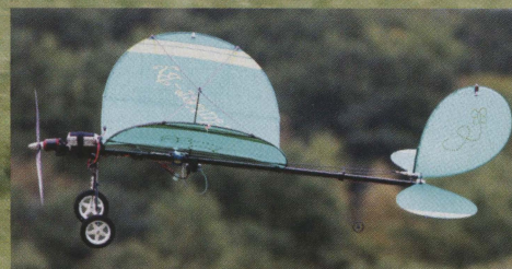
The "Flutter-By" is flown by Jack Frost and has a wingspan of 39 inches and weighs 18 ounces.
